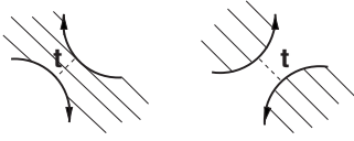
FIG. 2. Action of the tunneling Hamiltonian for a contact that is almost open (left) and for one that is almost pinched off (right); the shaded region is occupied by electrons.
