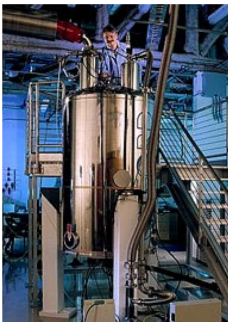
Figure 1. Pacific Northwest National Laboratory's high magnetic field (800 MHz, 18.8 T) NMR spectrometer. (Woodley, 2010)
